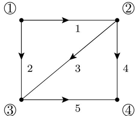
**Example 3.** Consider the graph to the right. Determine its edge-node incidence matrix  $M$ .
